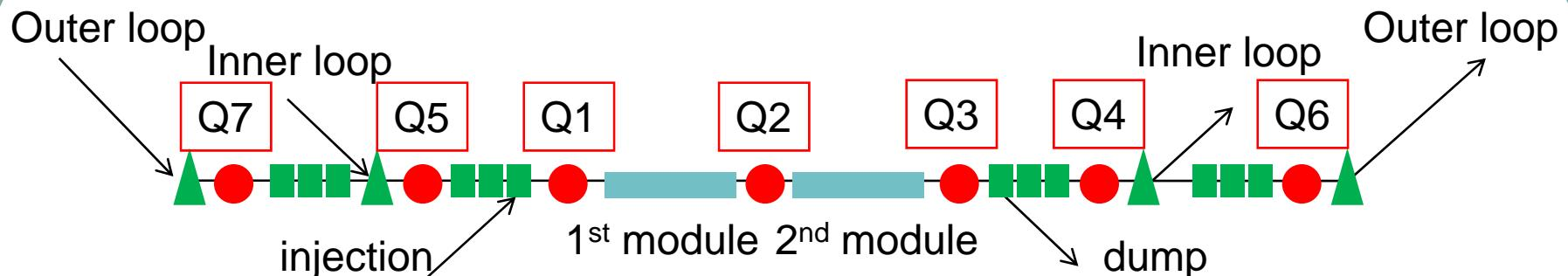
Beam energy at each quad (5 MeV injection, 60 MeV linac)
