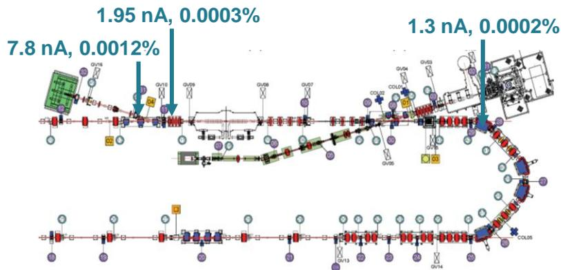
Calculated for total beam current 300  $\mu\text{A}$ \*\*
