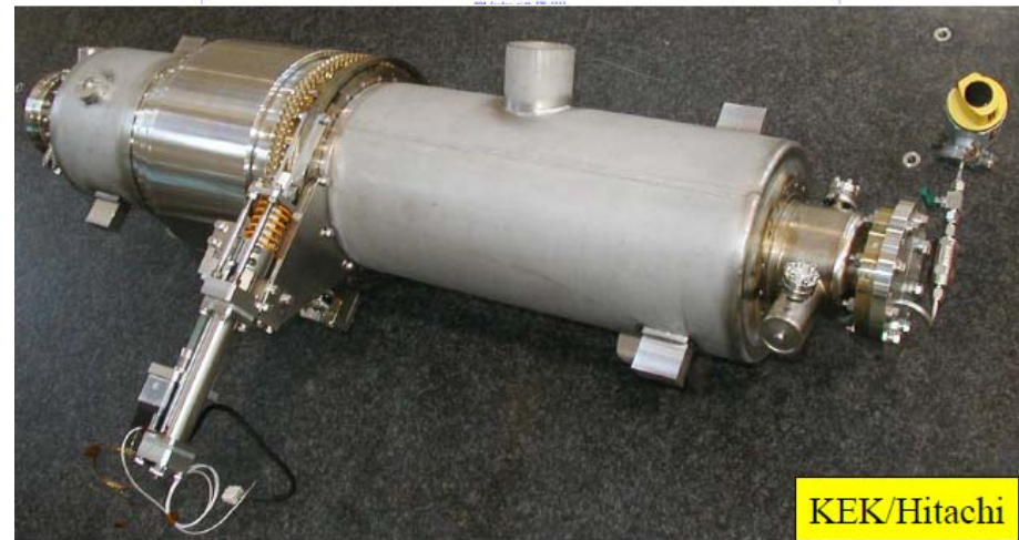
Input Coupler using capacitive coupling
