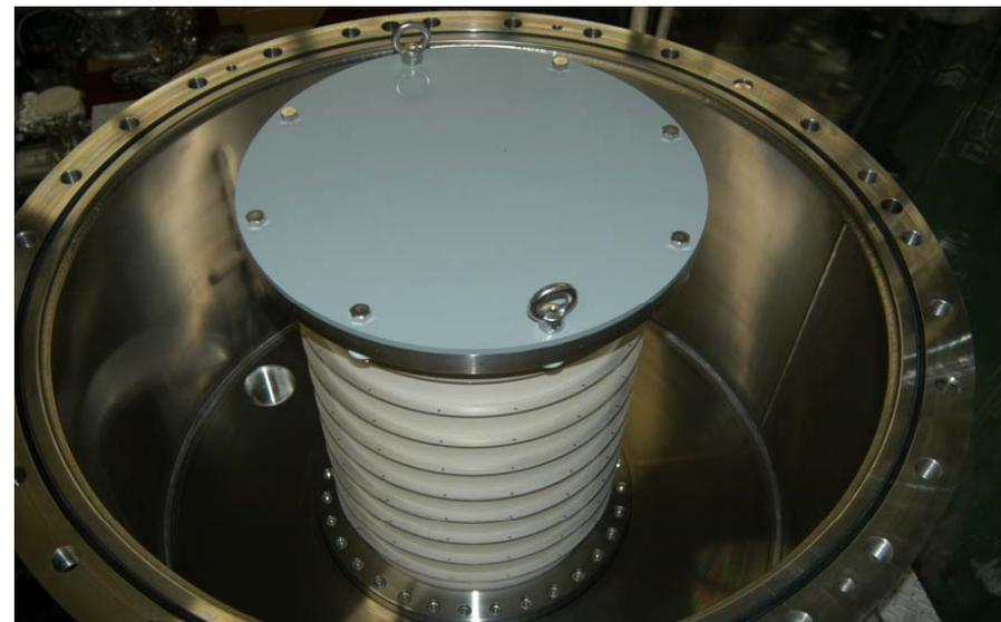
1. Assembly of guard rings and HV chamber.
