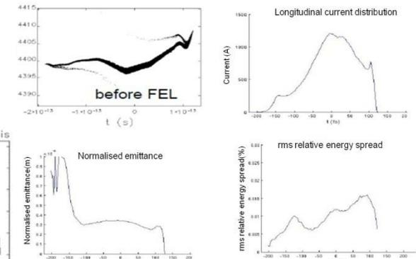
Tracked 100k particles. The data is binned in 1fs slices.
