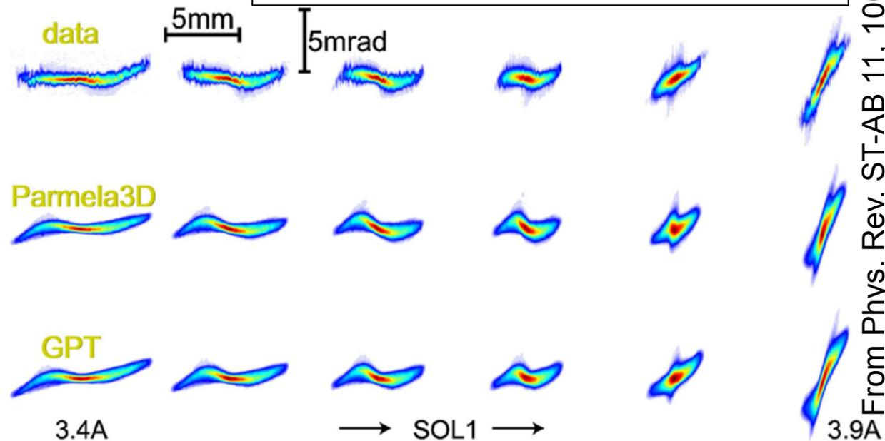
Are transported through the accelerator, measured in a fixed slit phase space measuring system, and compared with simulations.
