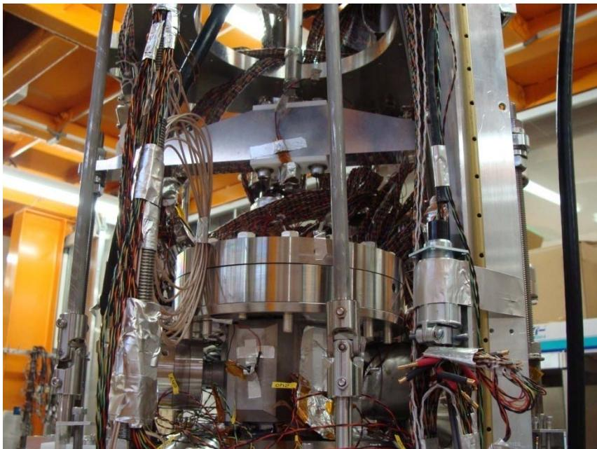
Variable input coupler was moved to bottom side, to avoid dust contamination from bellows
