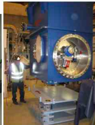
SRF gun In cryomodule
