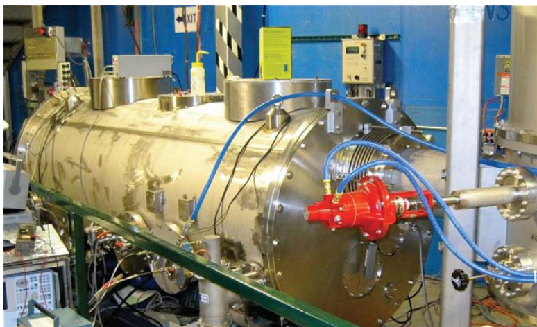
HTC: Horizontal Test Cryomodule
