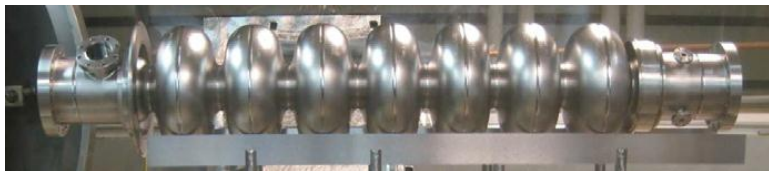
First Nb prototype cavity for ML(7-cell)
