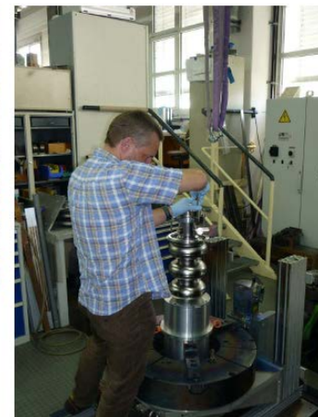
EB welding of helium vessel parts to finished cavity Cavity inner surface is already cleaned to ISO4 standards and sealed to ambient during EB operation
