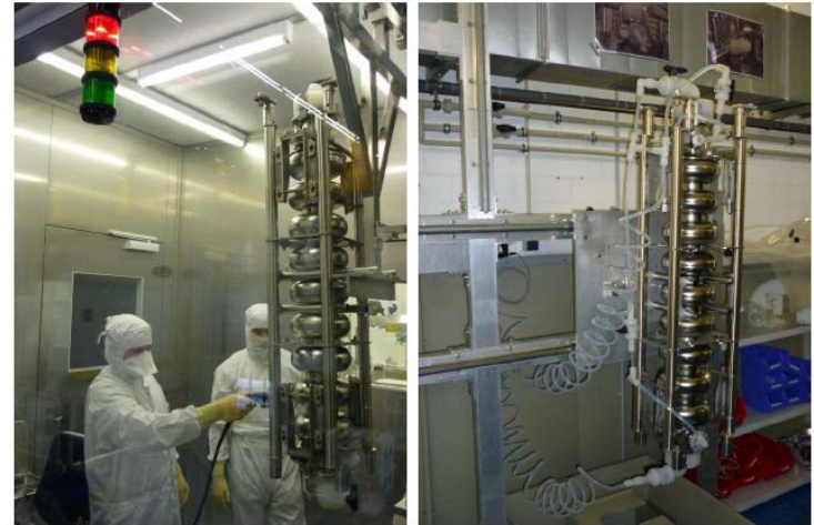
Cleaning of outer and inner surface of cavity prior entering ISO4 clean room
