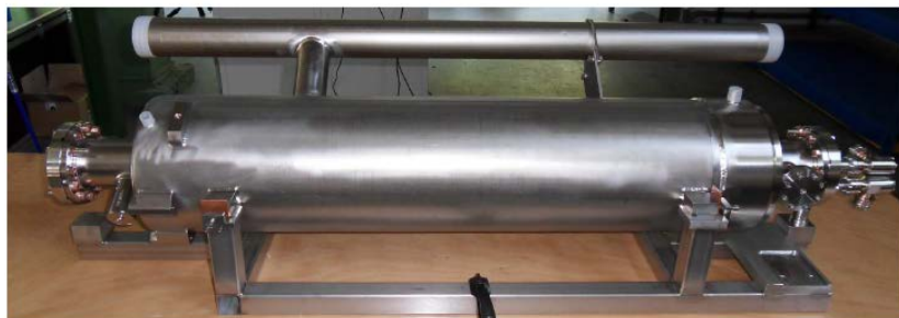
XFEL cavity after helium vessel welding
