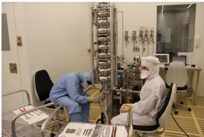
Assembly and leak checking in ISO4 clean room, A new 160 m 2 ISO 4 clean room was installed for the XFEL production
