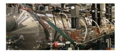
4 MeV, 75 mA CW beam accelerated by SRF cavities
