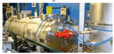
Q<sub>0</sub>=1·10<sup>11</sup> at 1.6K, 16 MV/m in a cryomodule
