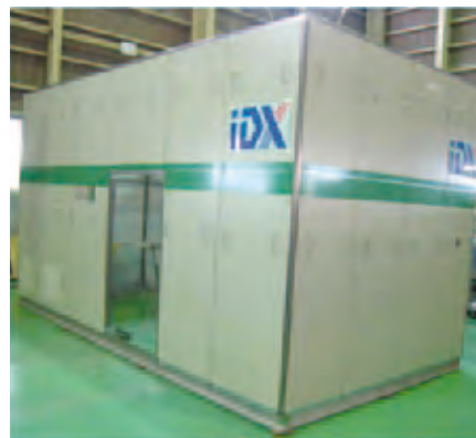
Figure 5-23 Photograph of the 300-kW klystron PS.
