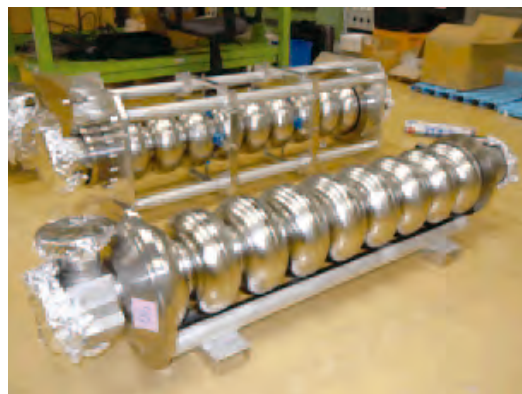
Figure 5-19 A pair of 9-cell cavities for the prototype module.
