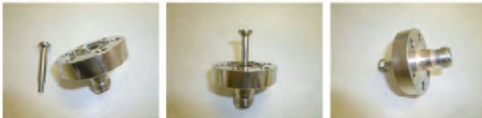
Figure 5-15 Development of new RF feedthroughs; Type-0 (left), Type-I (center) and Type-II (right).
