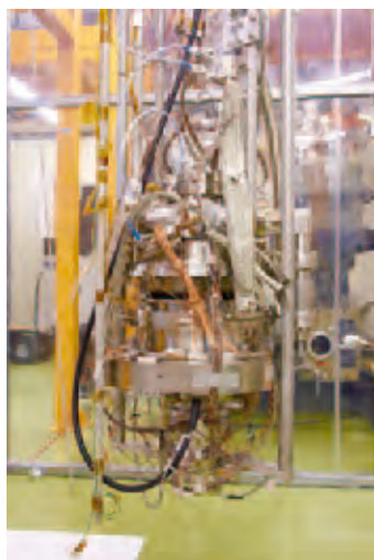
Figure 5-13 Set-up of vertical test of 2-cell cavity (left), and Q_0 – E_{acc} plots in the first test of the 2-cell #3 cavity (right).
