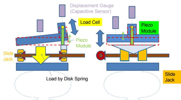
Figure 3: Piezo tuning system.
