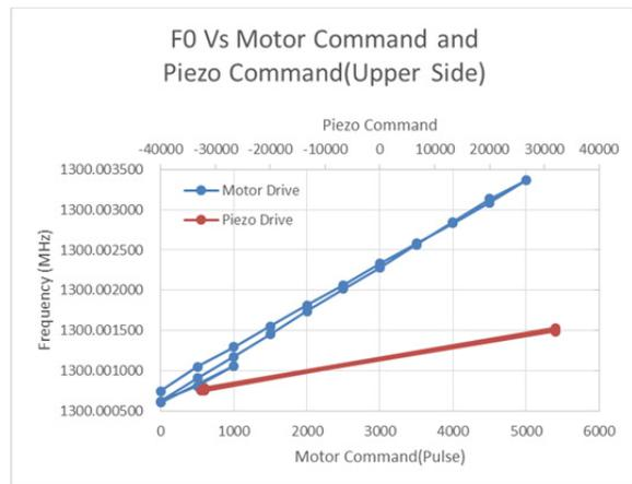
Figure 6: F0 vs motor command and piezo command.
