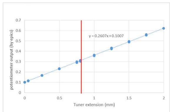
Figure 7: Amplitude vs potentiometer.
