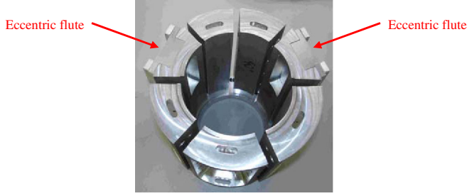
FIG. 5. (Color) Angularly divided eccentric-fluted beam pipe.
