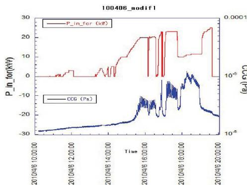
Figure 7: Results of high power test of new ceramic window. Left (right) axis shows the P\_in\_for (vacuum pressure).
