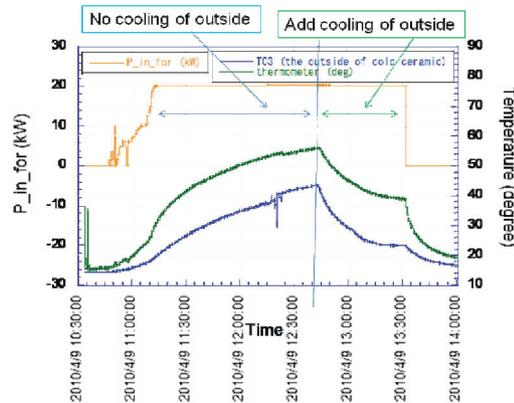
Figure 8: Results of high power test of new ceramic window. The left axis shows the P\_in\_for. The right axis shows the temperature of ceramic window measured by the thermometer (green line) and the outside of ceramic window (blue line).
