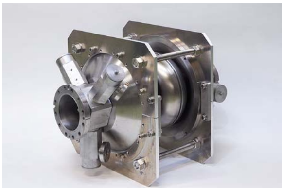
Figure 2: The second prototype cavity for the injector.
