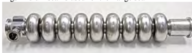
Figure 2 : Prototype of KEK-ERL model-2 cavity.
