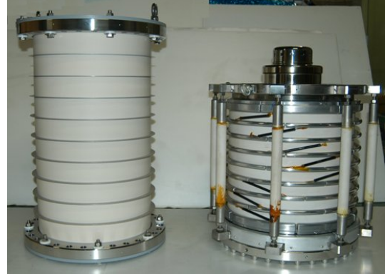
Figure 2: Multi-segmented ceramic insulator tubes for the old 250-kV JAERI FEL gun (right) and the 500-kV ERL gun (left). The guard rings are not installed at the 500-kV insulator.
