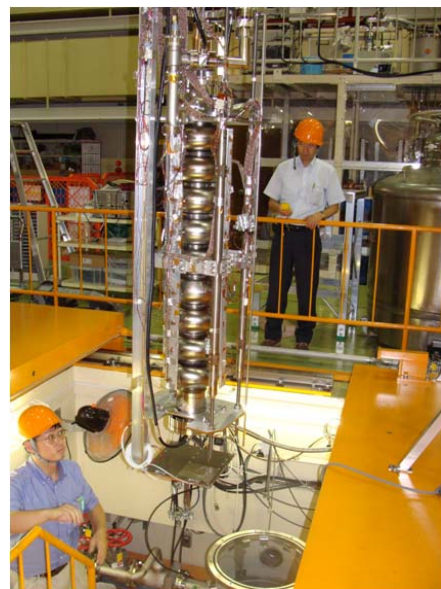
Figure 3: Preparation for the vertical testing the 9-cell cavity.
