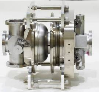
1.3GHz 2-cell Cavity 7.5 MV/m x 3 → 5 MV
