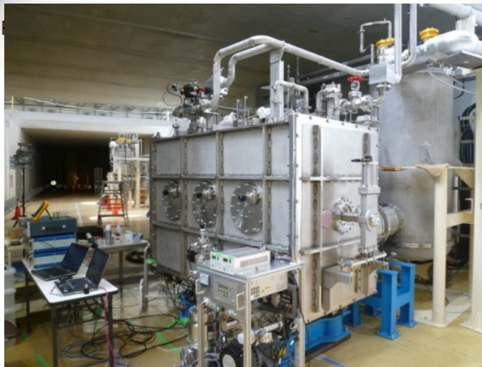
1.3GHz 2-cell Cavity 7.5 MV/m x 3 → 5 MV
