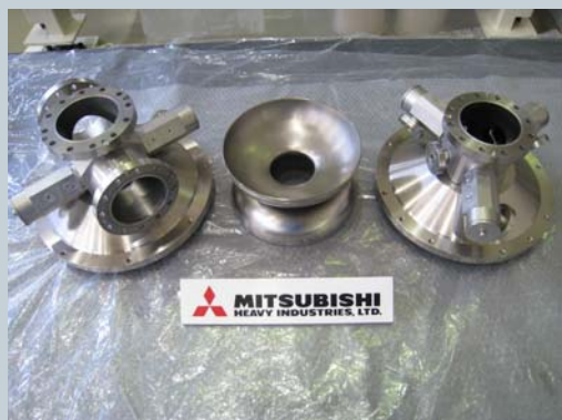
ERL 2-cell #3, #4, #5 Cavity under fabrication
