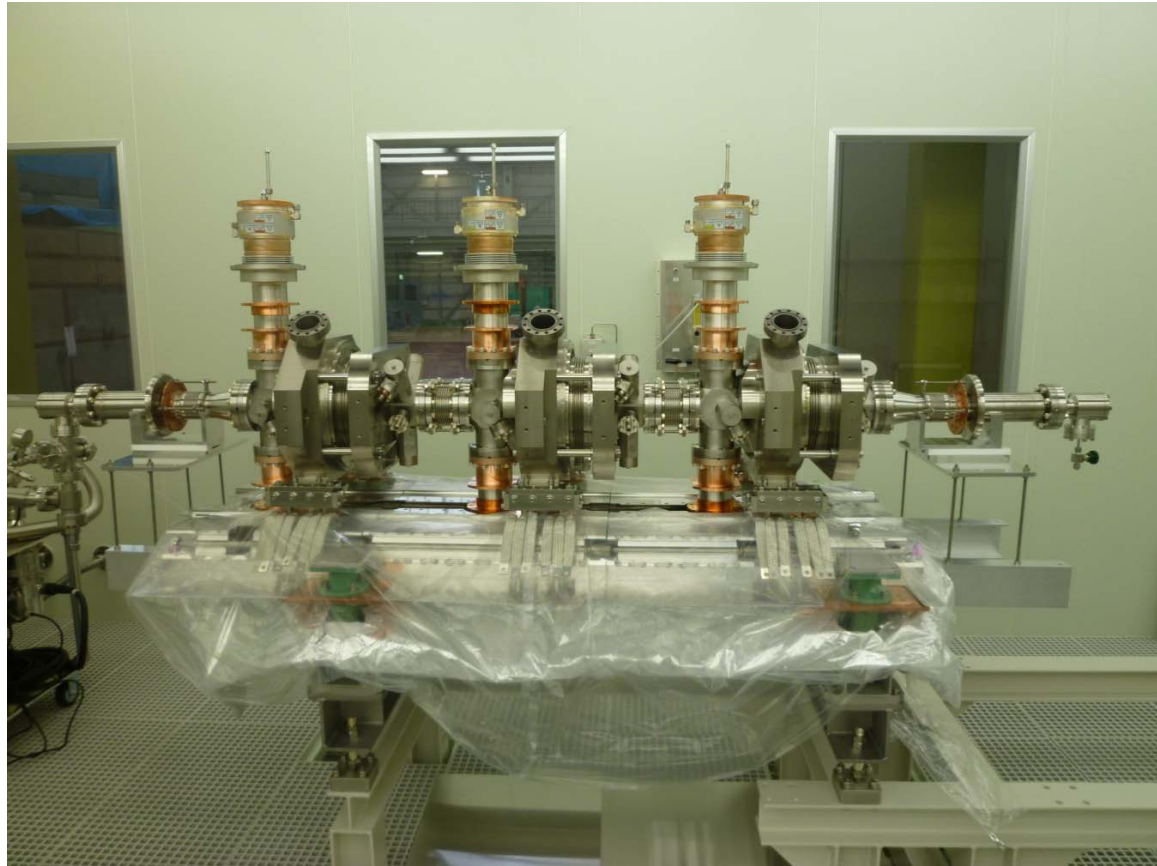
Cavity string assembly in clean room
