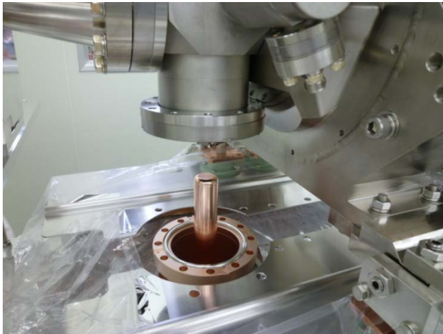
Attachment of input couplers
