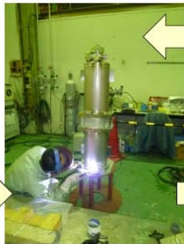
TIG weld of He Jacket at CFF
