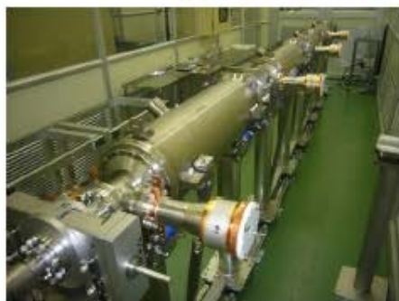
Cavity string assembly 1 week
