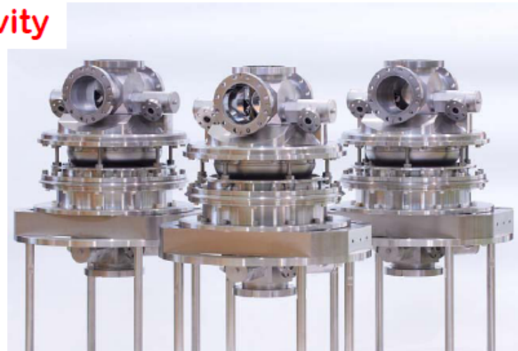
Three 2-cell cavities with 5 HOM couplers
