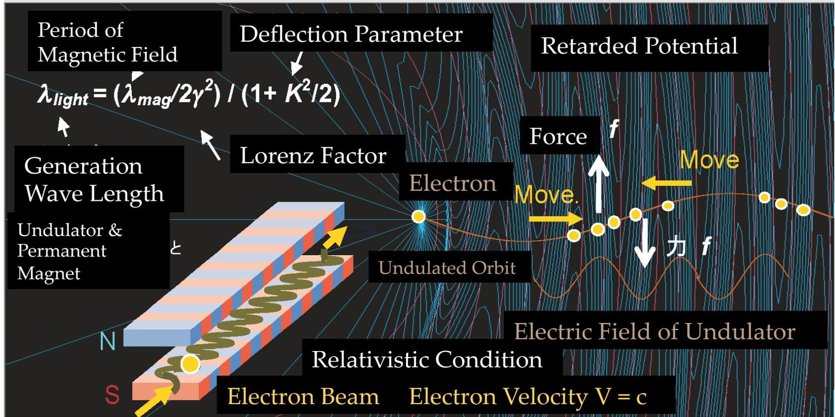
COHERENT SYNCHROTRON RADIATION
