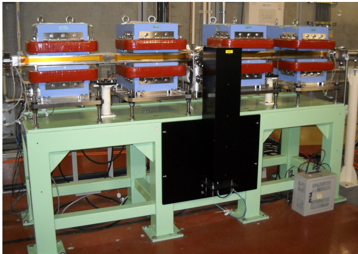
CERL chicane for path-length control
