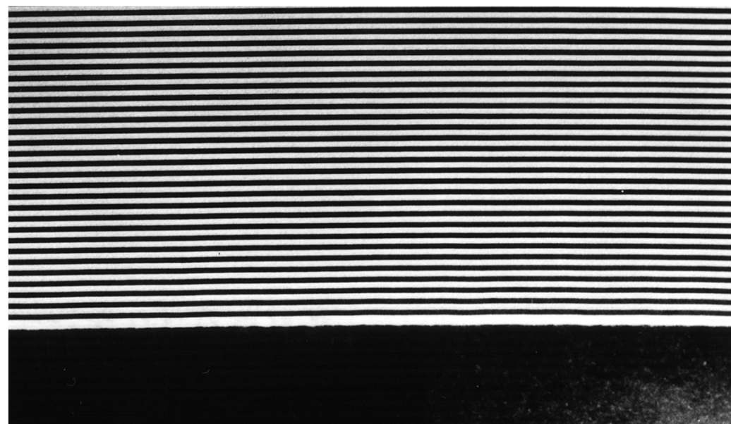
TEM cross sectional TEM image of Mo/SiC multilayer
