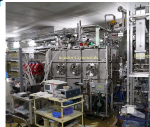
2-cell SRF cavity for cERL cERL injector cryomodule
