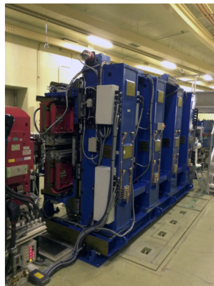
Figure 4: Photograph of the new undulator installed at BL-28.
