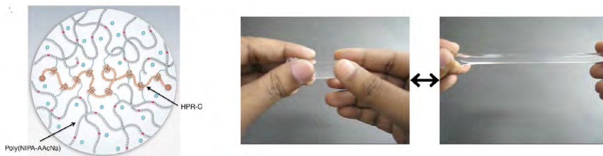
Figure 1: Schematic view of highly stretchable hydrogel containing polyrotaxane cross-linkers and photograph of deformed state of the gel. The figure was reproduced from ref. 4.
