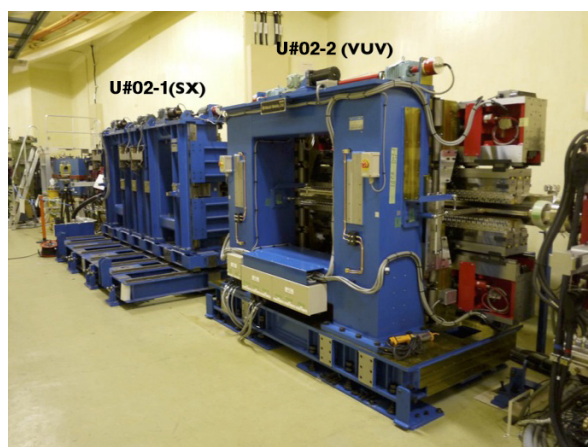
Figure 1: Photograph of two undulators U#02-1 (for SX) and U#02-2 (for VUV) for BL-2.
