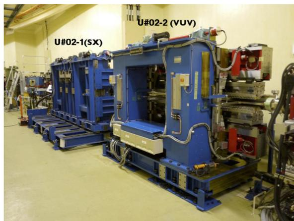
Figure 1: Photograph of two undulators U#02-1 (for SX) and U#02-2 (for VUV) for BL-2.
