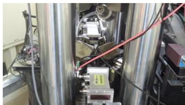
Fig. 2: A close view of the sample stage from the incident-beam side. The IC on this side is I_0 in Fig. 1, and the IC on the other side is I . Anvil blocks are seen between the two ICs.
