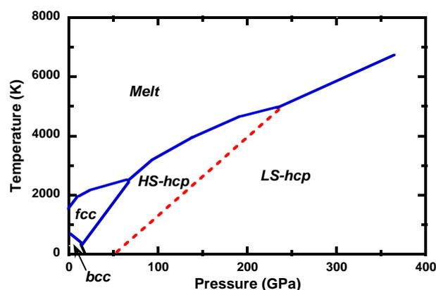
Fig. 1: Schematic phase diagram of iron at high pressures and temperatures. The dashed line represents the boundary between the high-spin (HS) and low-spin (LS) states in hcp-Fe.
