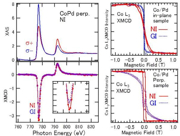
Fig. 1, XAS and XMCD of Co  $L$ -edge in perpendicularly magnetized Co (0.69 nm)/Pd (1.62 nm) multilayer. Inset shows the expanded view of  $L_3$ -edge XMCD. Element-specific hysteresis curves at Co  $L_3$  edge for PMA and in-plane samples are also shown.
