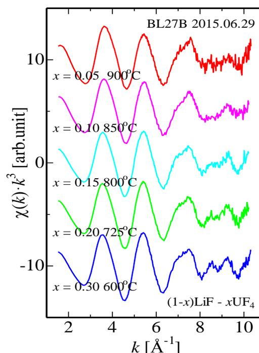
Fig. 1 EXAFS oscillations of LiF-UF<sub>4</sub> ( $x_{\text{UF}_4} = 0.05, 0.10, 0.15, 0.20, 0.30$ ) at molten phase.
