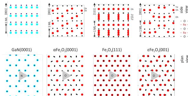
Fig. 1: Lattice matching between GaN(0001),  $\alpha\text{Fe}_2\text{O}_3$  (0001),  $\varepsilon\text{Fe}_2\text{O}_3$  (001),  $\text{Fe}_3\text{O}_4$  (111) and  $\gamma\text{Fe}_2\text{O}_3$  (111).
