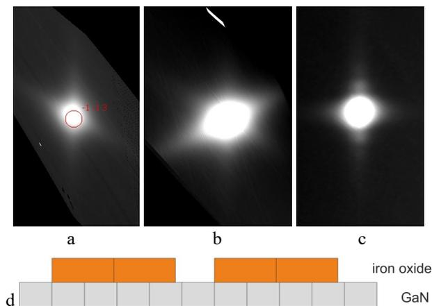
Fig. 3: Off-specular XRD maps. Reciprocal space cuts parallel to the surface showing star-like shapes of  $\epsilon\text{Fe}_2\text{O}_3$  (113) (a) and  $\epsilon\text{Fe}_2\text{O}_3$  (112) (b) reflections. Reciprocal space cut perpendicular to the surface showing the Laue oscillations on the streak passing through  $\epsilon\text{Fe}_2\text{O}_3$  (112) reflection (c). Schematic explanation of stacking fault formation principle (d).
