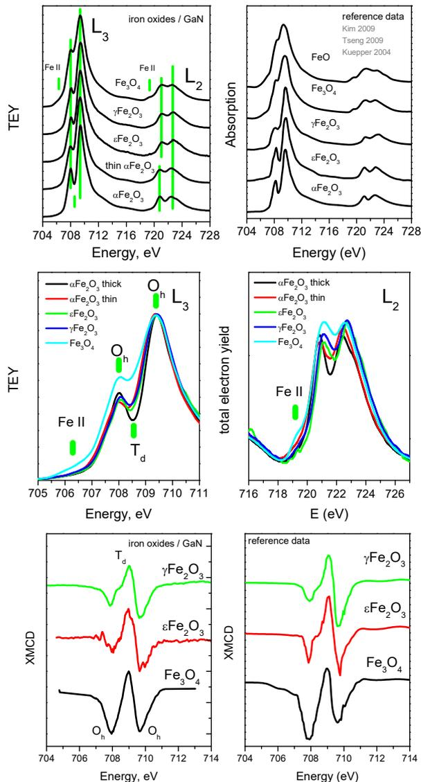
Fig. 4: XAS and XMCD spectra obtained from the iron oxide epitaxial films on GaN. Reference data adopted from [8,9,10] is shown for comparison.
