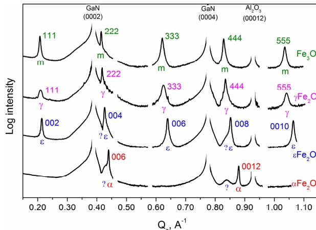
Fig. 2: XRD specular intensity profiles measured in epitaxial iron oxide layers on GaN(0001).
