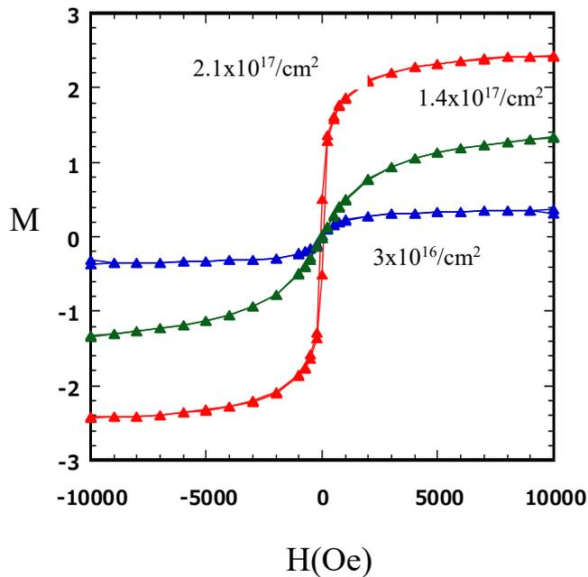
Fig. 2 Magnetization-external magnetic field ( $M$ - $H$ ) curves for silica glass samples Fe-implanted with fluences of  $3 \times 10^{16}$ ,  $1.4 \times 10^{17}$  and  $2.1 \times 10^{17}/\text{cm}^2$ .
