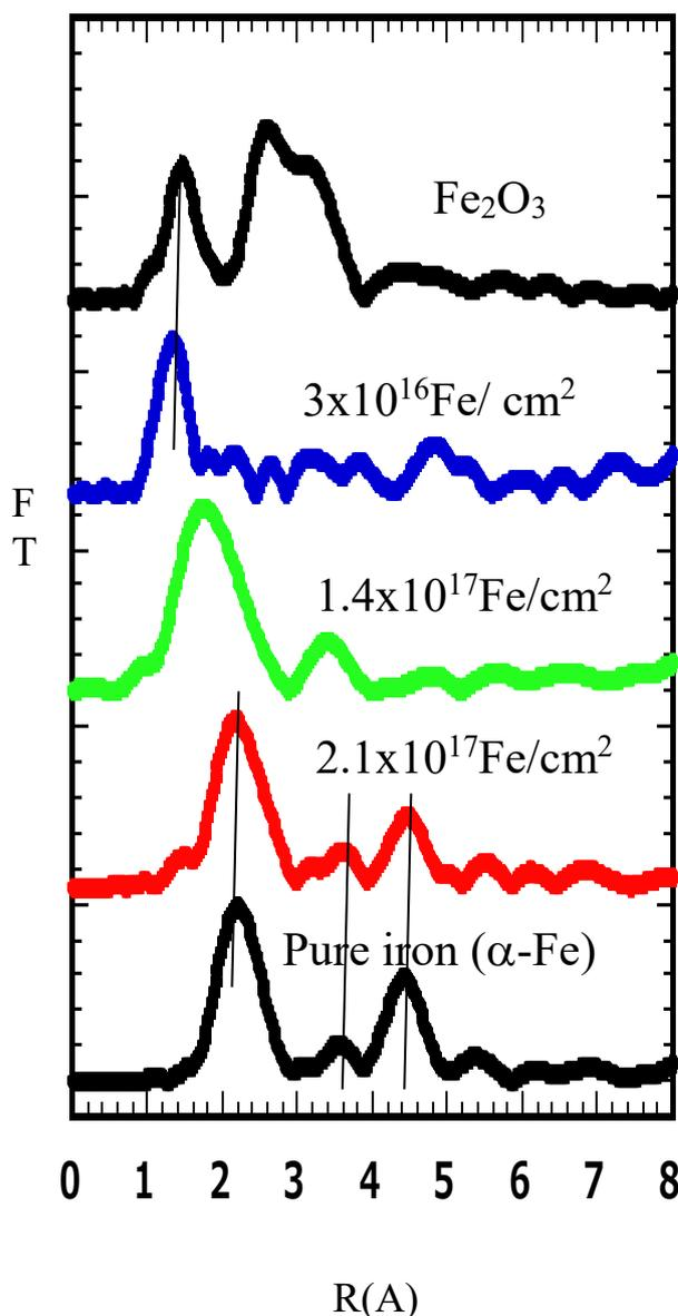
Fig. 1 EXAFS-FT spectra for silica glass implanted with Fe ions. Spectra for Fe<sub>2</sub>O<sub>3</sub> and pure iron are also shown.
