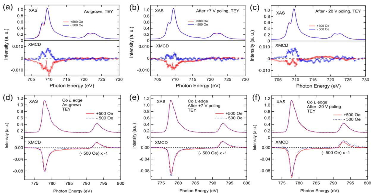
Figure 2. XAS and XMCD spectra at the Fe and Co  $L_{3,2}$ -edges of Co/BFO heterostructure. (a) Fe  $L_{3,2}$  edges at the as-grown state, (b) After a +7 V voltage poling, (c) After -20 V voltage poling. (b)-(d) Co  $L_{3,2}$  edges under the same condition as Fe.
