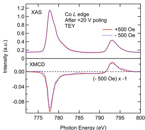
Figure 4. XAS and XMCD spectra at the Co  $L_{3,2}$  edge after a +20 V voltage poling.
