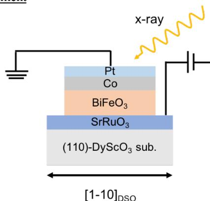
Figure 1. Setup for the voltage-dependent XAS and XMCD measurements.
