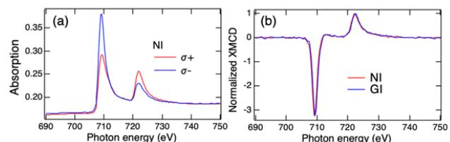
Fig. 2 (a) Fe- $L_{2,3}$  edges absorption spectra in NI and (b) XMCD in Fe(0.7 nm)/W(0.15 nm)/MgO(2 nm).
