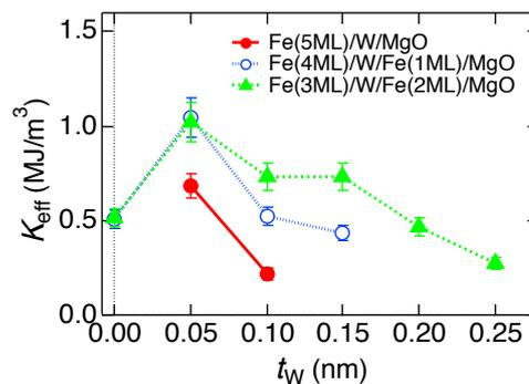
Fig. 1  $K_{\text{eff}}$  values depending on  $t_{\text{W}}$  by magnetization measurement. Each line indicates the position of W in Fe/MgO interfaces.
