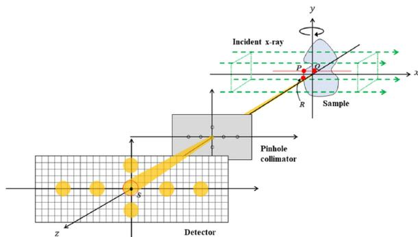
Fig. 1: Schematic of mp-XFCT
