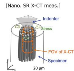
Fig. 1 Schematic image of the part of the CFRP specimen for the nanoscopic SR X-CT measurements [2].
