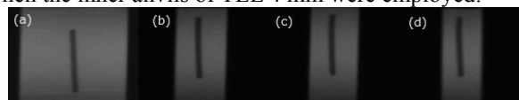
Fig. 2: A transmission image of the dummy sample in an anvil gap when a POM frame was employed is shown. (a) Anvil gap 2.11 mm at ambient conditions, (b) 0.99 mm at 5.0 GPa and room temperature, (c) 0.94 mm at 3.0 GPa and 1500 K, and (d) 0.78 mm at 5.8 GPa and 1500 K.
