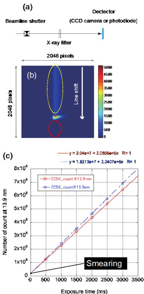
Fig. 2: Calibration of an x-ray CCD camera. (a) is experimental setup. (b) is a typical image recorded by the CCD camera. (c) indicates the count number of the CCD cameras as function of the exposure time for the wavelength of 13.9 nm.
