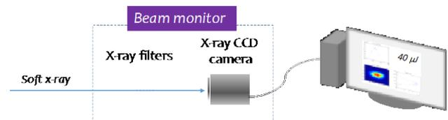
Fig. 1: Schematic view of the CCD-based energy monitor
