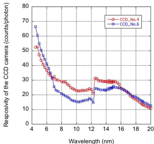
Fig. 3: The sensitivity curves of x-ray CCD cameras.
