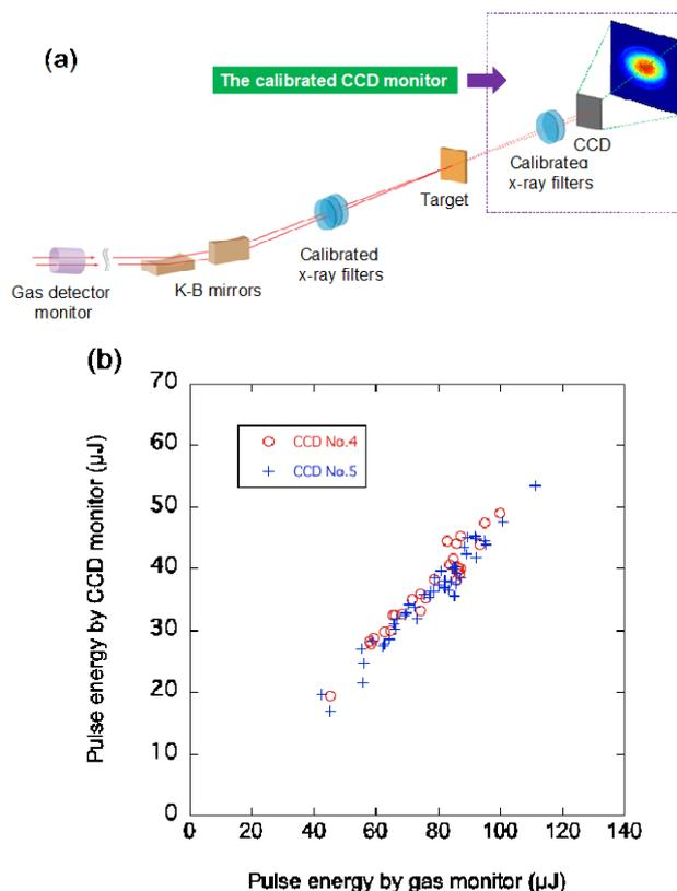
Fig. 5: Operation of the CCD-based energy monitor in an application study at the SACLA SXFEL. (a) Schematic view of the damage test experiment. (b) indicates the linearity of the CCD-based energy monitor versus the gas detector monitor which has been installed at the SACLA SXFEL.
