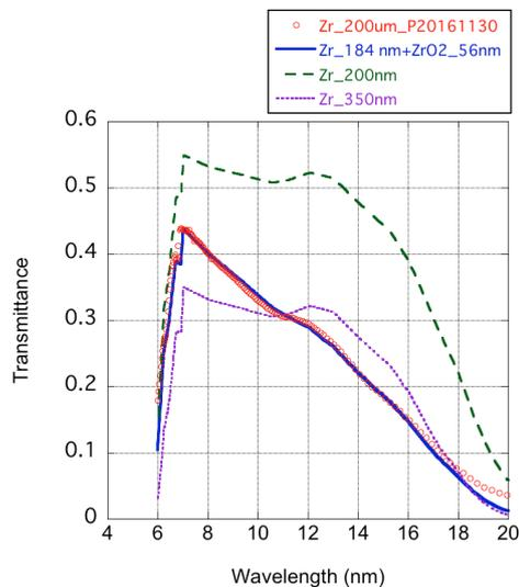
Fig. 4: Transmittance of a Zr filter with a nominal thickness of 200 nm. The red circles is the measured value. The green-dashed-line and purple dotted-line are the transmittance of Zr filters calculated from the data base for the thickness of 200 nm and 350 nm, respectively. The solid-blue-line is the calculated curve with the thicknesses of Zr and ZrO<sub>2</sub> layers of 184 nm and 56 nm, respectively.
