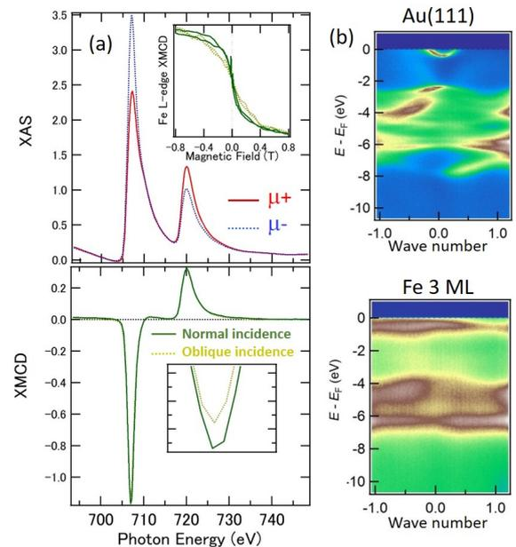
Fig. 1, XAS and XMCD of Fe *L*-edges in 3-ML-thick Fe on Au(111). (a) XAS in normal incidence and XMCD in both normal and oblique incidence cases. Insets show the M-H curves at Fe *L*<sub>3</sub> edge and expanded view around *L*<sub>3</sub>-edge. (b) ARPES of Au(111) surface and 3-ML-thick Fe deposited surface.
