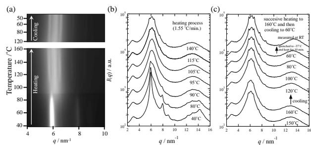
Fig. 1: (a) Changes in the one-dimensional WAXS profiles in the heating process and the subsequent cooling process. The panels (b) and (c) highlight the WAXS profiles in the heating and subsequent cooling processes.
