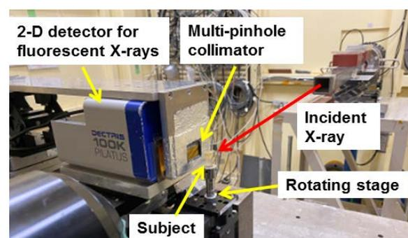
Fig. 1: Ultra-high-resolution multi-pinhole XFCT system.
