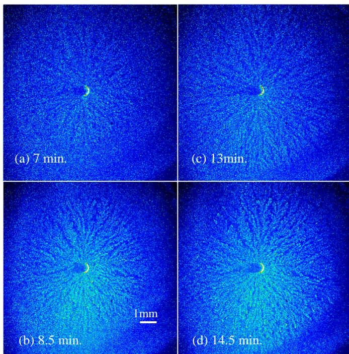
Fig. 1 XRF images obtained during the electrodeposition: (a) and (c) 9.3 keV irradiation (below Zn K-edge), (b) and (d) 9.8 keV irradiation (above Zn K-edge). Exposure time for each image is 1 min.
