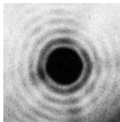
Fig. 1. Fraunhofer diffraction pattern of 1.39 Å X-rays from a 5 mm f pin-hole recorded on the photoplate set 1010 mm apart from the pin-hole.
