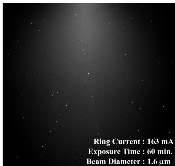
Figure 6. Micro-area Laue diffraction pattern of Ca silico-phosphate.
