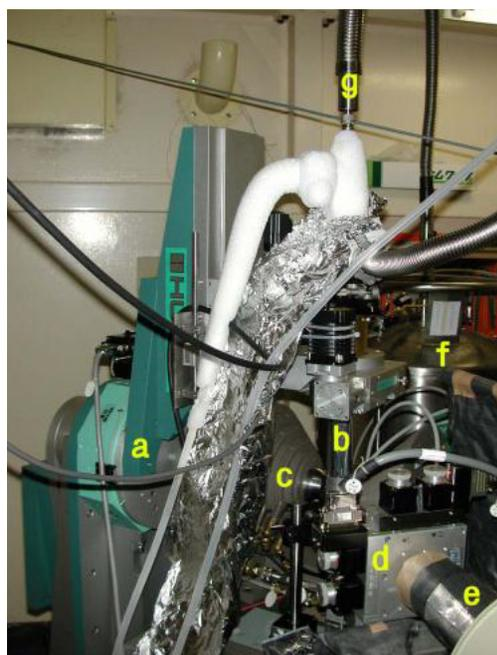
**Figure 3.** Experimental setup of the white X-ray magnetic diffraction of  $\text{YTiO}_3$ : a, five-circles diffractometer; b, refrigerator of liquid He-flowing type to keep the temperature of the specimen at 5 K; c, electromagnet producing 0.3 tesla at a gap length of 50 mm; d, slit for receiving diffraction beam and minimizing fluorescent radiation from the specimen; e, pure Ge solid state detector; f, vessel of liquid He; g, transfer tube of liquid He.
