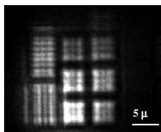
Fig. 2. X-ray image of a test pattern with lines and spaces of defined widths taken at 1.5 nm.
