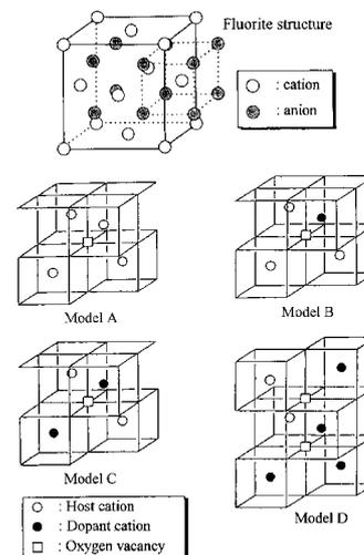
Fig. 2. Four models showing the local structures around vacancies.
