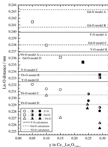
Fig. 1. Comparison of the calculated lines of the average Ln-O inter-ionic distances and the experimental Ln-O distances in  $Ce_{1-x}Ln_xO_{2.00-y}$ . Each of open, half-filled and filled symbols stands for the data of non-reduced, reduced and quenched samples, respectively.
